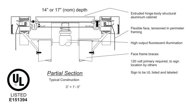
Reference: Series 250-UL DF Illuminated Flex-face Sign Standard Specifications, Outboard Mount
