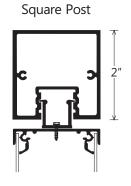
Removable Post Caps Allow panels to slide up and out of posts 0", 3/8", 3/4"
