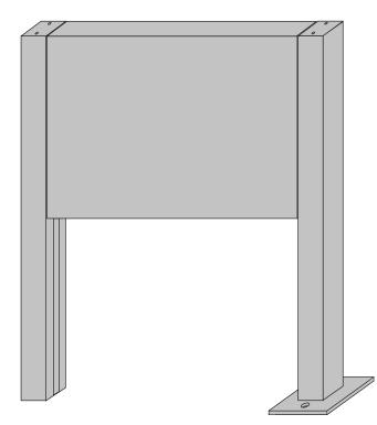
Non-illuminated Variable size, up to approx. 50 sq. ft. 3-1/4" deep panel with flush .090" aluminum faces 3-1/4" square, rectangular or half-round posts Optional reveal at post to panel connection Baked 2-part acrylic polyurethane finish Direct burial or base-plate mounting
